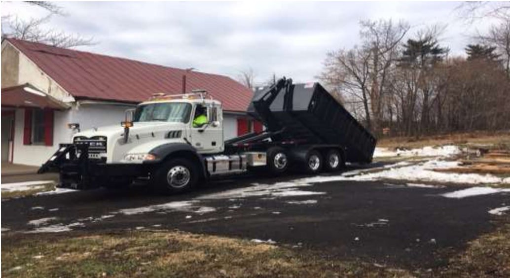
Mack Hook Truck for Public Works
